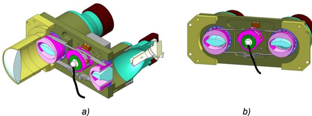
*Figure 3 a) Appearance of the headlamp in section
