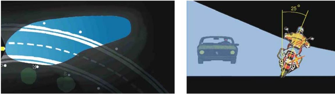
*Figure 1 Visibility and passing track with oncoming vehicle when using headlamp without adjusting gadget*
