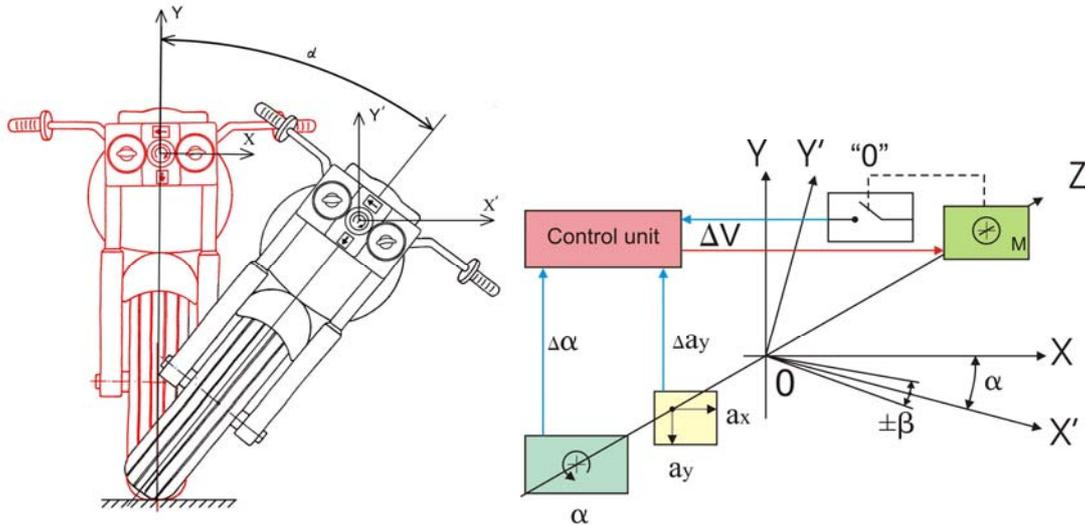
Fig. 7. Diagram of operation of the adjusting system
