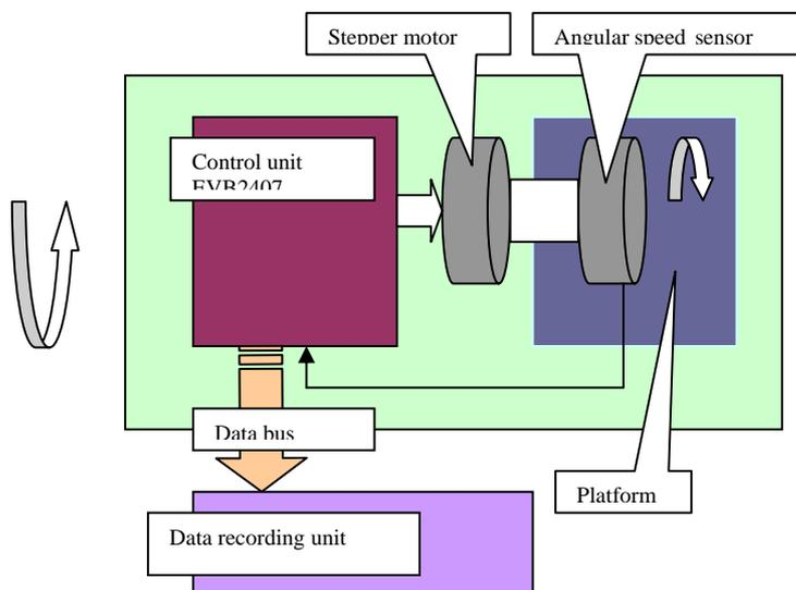
*Fig. 6. The block diagram of the adjusting module*
