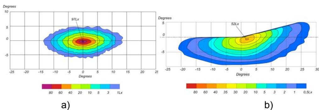
*Figure 4 a) High beam light pattern with H7 bulbs
