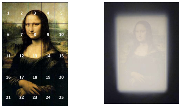
Figure 7. The light measurements on the painting show a uniformity of 0.85 (with the lamp alone) and 0.92, taking the ambient light into account.
